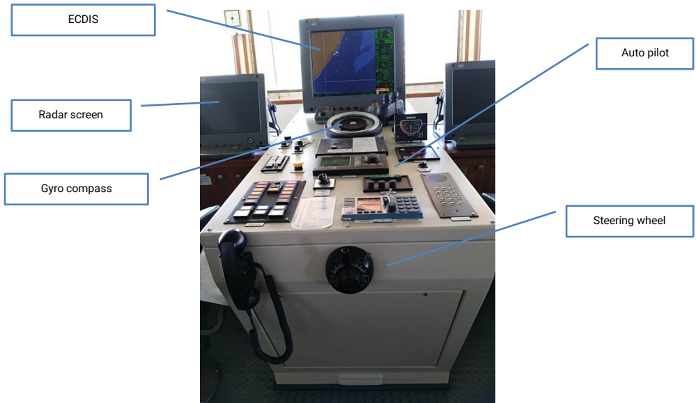
Figure 12: The auto pilot console with steering wheel and gyro compass repeater.
