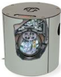
Figure 9: Gyrocompass - the sphere with gyroscope
