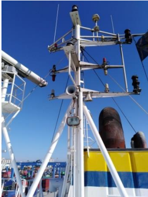
Figure 55: Mast of a cargo vessel with the navigation lights.
