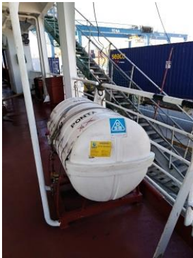
Figure 38: Cylindrical container holding a life raft.
